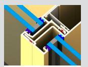
Full width interlocking legs both sides of glazing pocket provides added strength and support for heavy double glazing up to 30mm.
