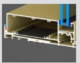
We recommend all commercial framing systems are installed with sub-sill. The sill is fixed to to sub-sill for improved performance under ultimate negative wind loads.
